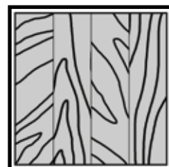
Random Matched Face Veneer slices are aligned in a random, but pleasing manner. Patterns are less likely to occur. Tight-side-out is possible. Veneer slices may be random in width as well.
